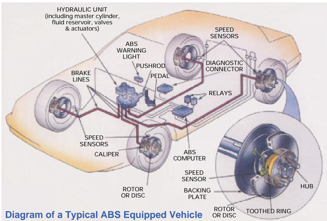
**Diagram of a Typical ABS Equipped Vehicle**
